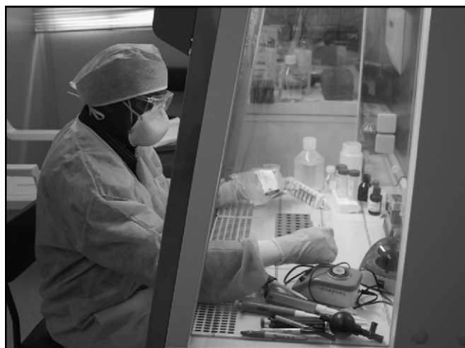
Fig. 4. Sample Processing in the Kenema Government Hospital Laboratory. Samples are manipulated in class II biosafety cabinets by personnel wearing full personnel protective materials. (Photo by Joseph Fair.)
